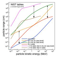
Figure 2: Range of radiation in air and
