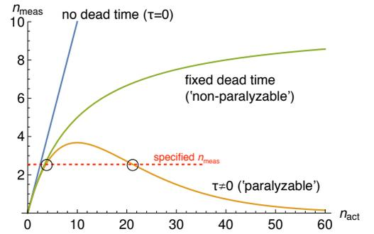
Figure 2: Schematic dependence of measured count rate on actual count rate (note switch of usual ordinate and abscissa) with no dead time (blue), a fixed dead time (green), and a fixed dead time in a paralyzable model. To find the actual count rate in the paralyzable case one must find the intersection of a specified measured rate with the orange curve.
