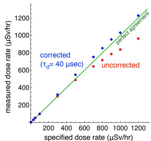
Figure 1: Redrawn data of WKC [1] for bGeigie Nano, red. Blue dots indicate correction for a fixed dead time of 40  $\mu\text{sec}$  and the green line indicates perfect agreement between measured and specified dose rates.
