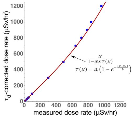
Figure 5: Correction curve including dose-dependence of the dead time extracted from WKC data.
