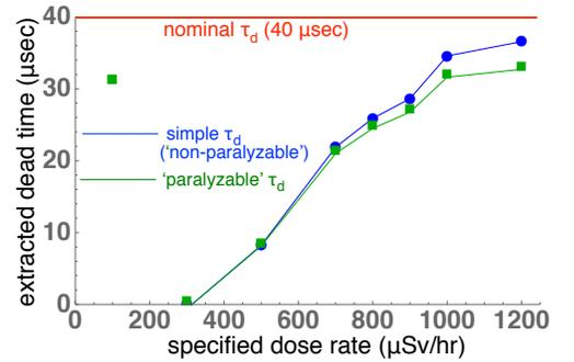
Figure 3: Evolution of the extracted dead time with specified dose rate in a non-paralyzable model (blue), in the paralyzable model (green). The fixed, nominal ‘minimum dead time’ for the Geiger-Müller tube is shown in red.
