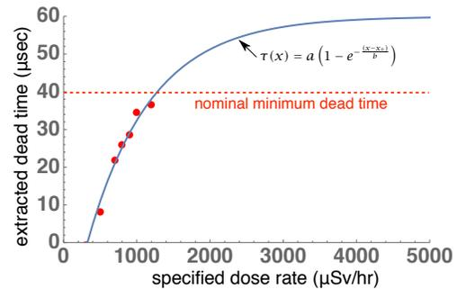
Figure 4: Fit to the dose rate dependence of the simple Geiger-Müller dead time extracted from WKC data.
